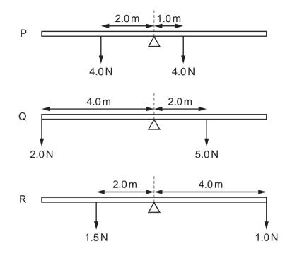
Which beams rotate clockwise?
